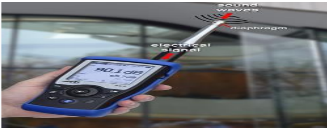
Figure 2: A Sound Level Meter, Is One of the Main Tools for Measuring Sounds in the Environment and the Workplace
