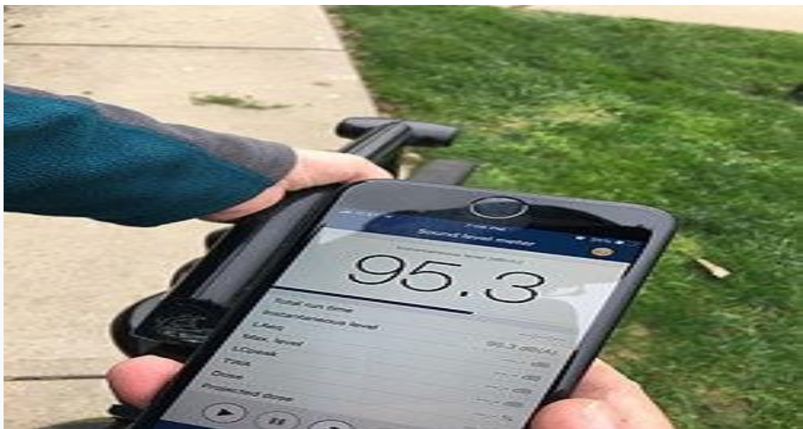
Figure 1: Noise Level from a Leaf Blower, using the NIOSH Sound Level Meter App
