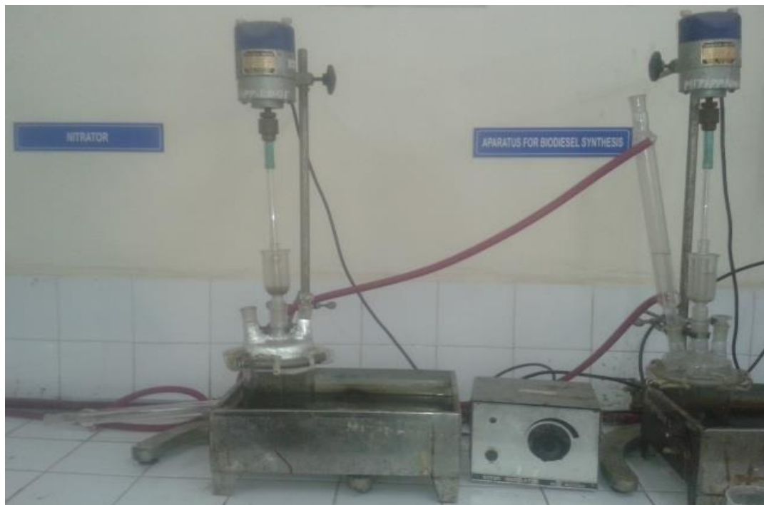
Figure 2: Experimental set up for Biodiesel Production in stirring method
